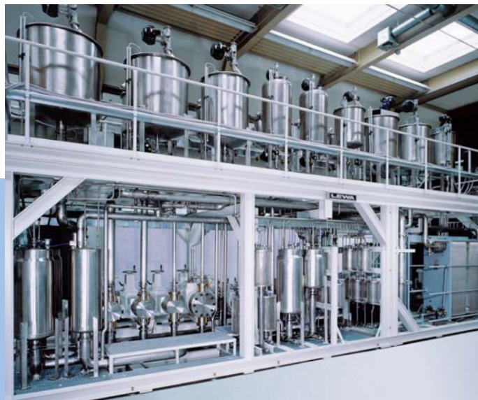
Complex systems for proportional blending or transfer of multiple product streams
