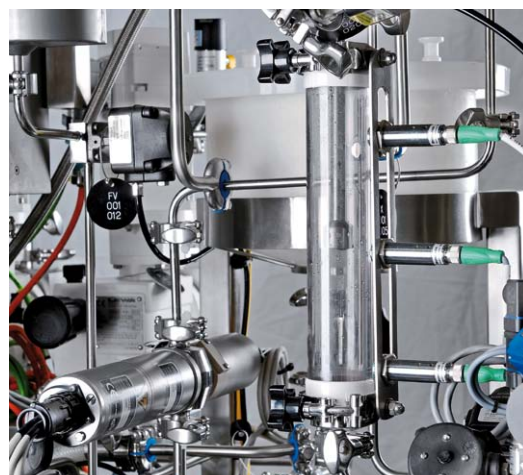
Bubble trap with level switches
