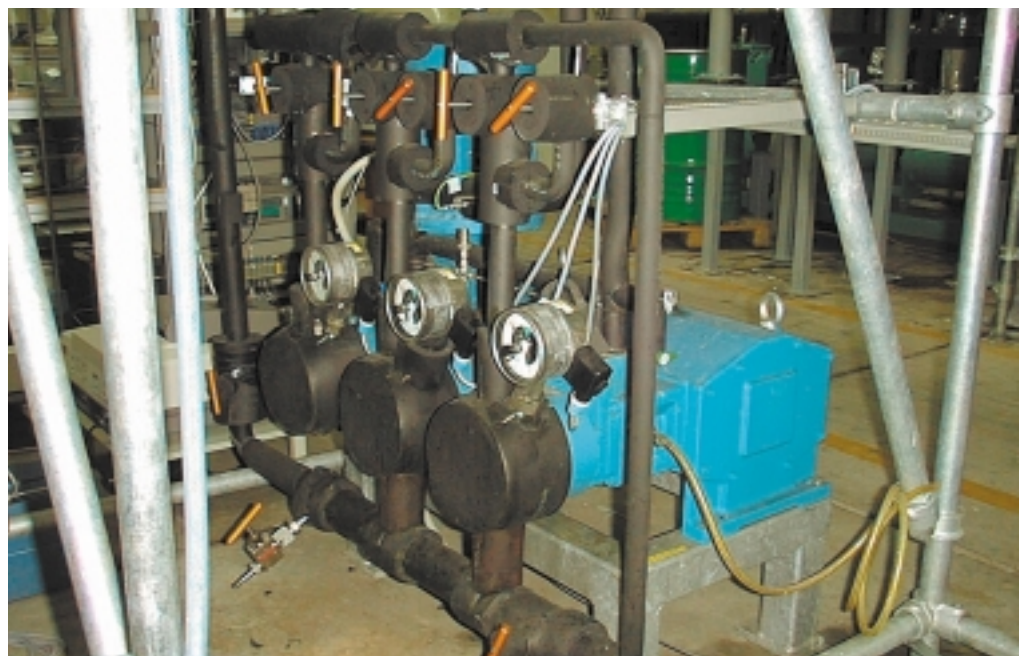
LEWA triplex diaphragm metering pump G3H in Mixer-Settler Extraction
