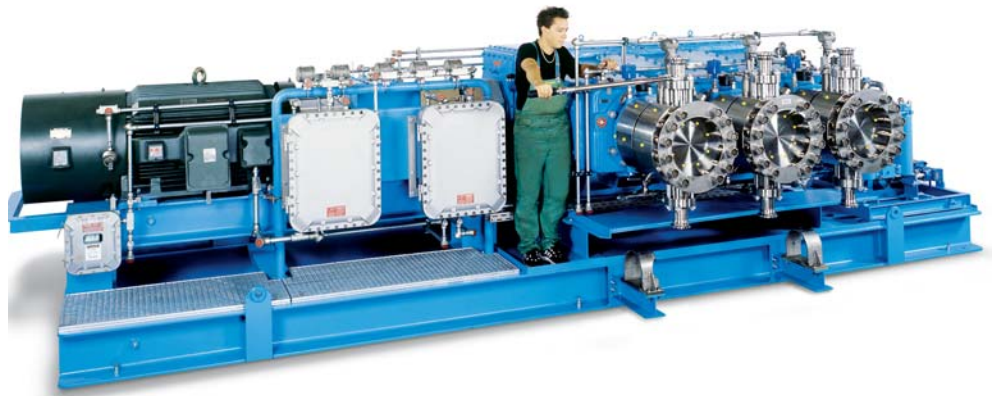
LEWA process-diaphragm pump G3U for H 2 S/CO 2 , 230 bar, 24 m 3 /h
