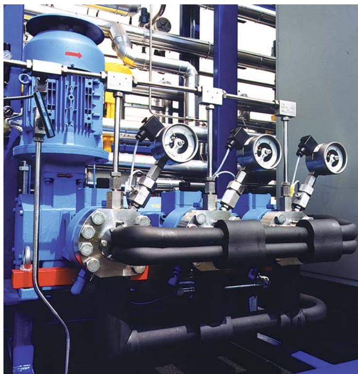
LEWA diaphragm pump for liquid CO 2 , with cooling device
