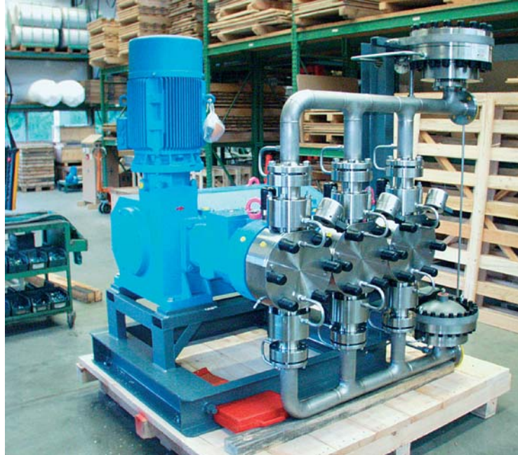
Fig. 1: LEWA triplex process diaphragm pump G3S for caprolactam melt
