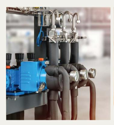
The metering of blowing agent is of particular importance to guarantee the constant quality of the end product in extrusion processes. LEWA ecofoam testing system has been designed for all known blowing agents, incl. cooling device for  $CO_2$  and explosion-proof design for combustible blowing agents.
